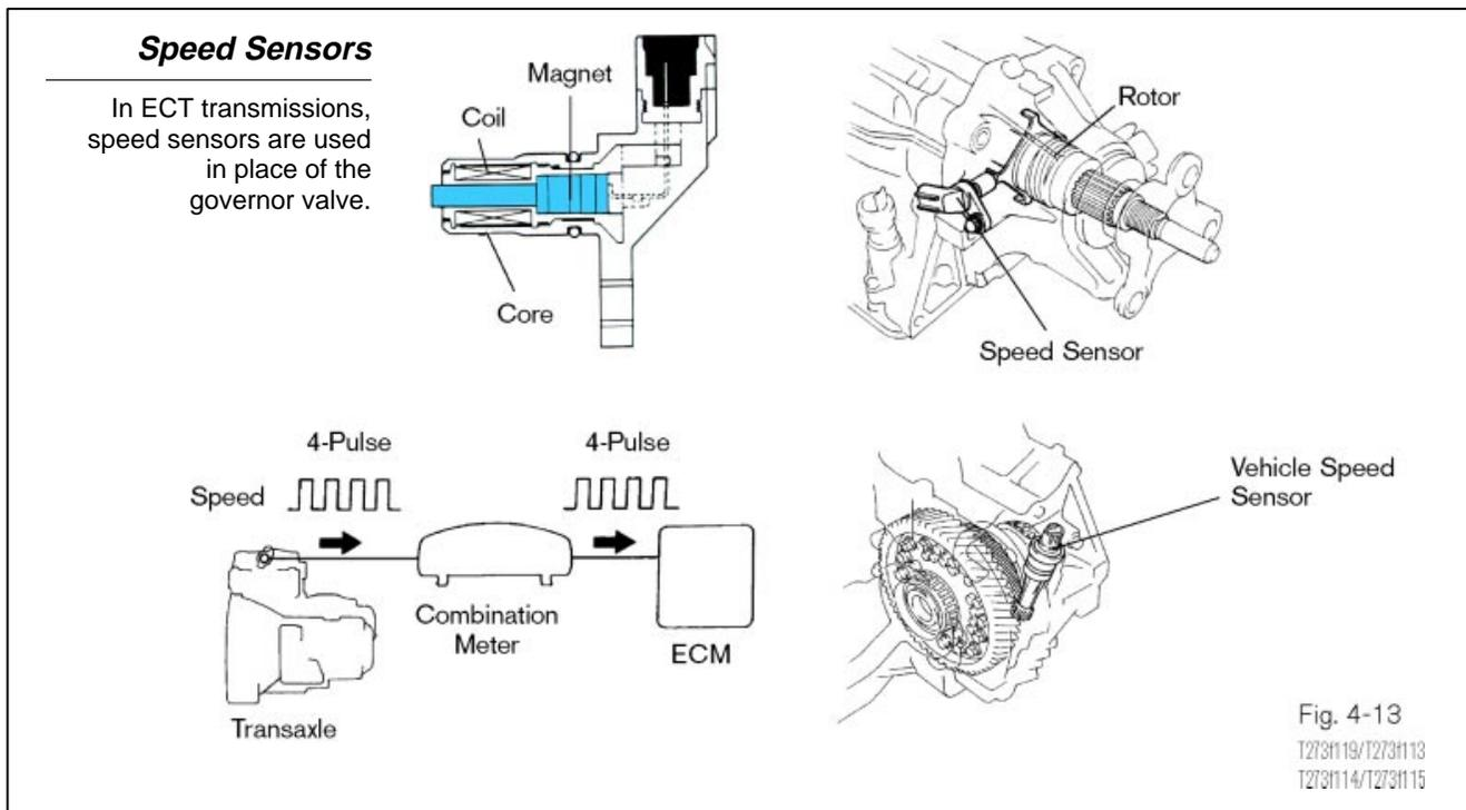
The distance between the rotor pickup coil is critical. The further apart they are, the weaker the signal.
