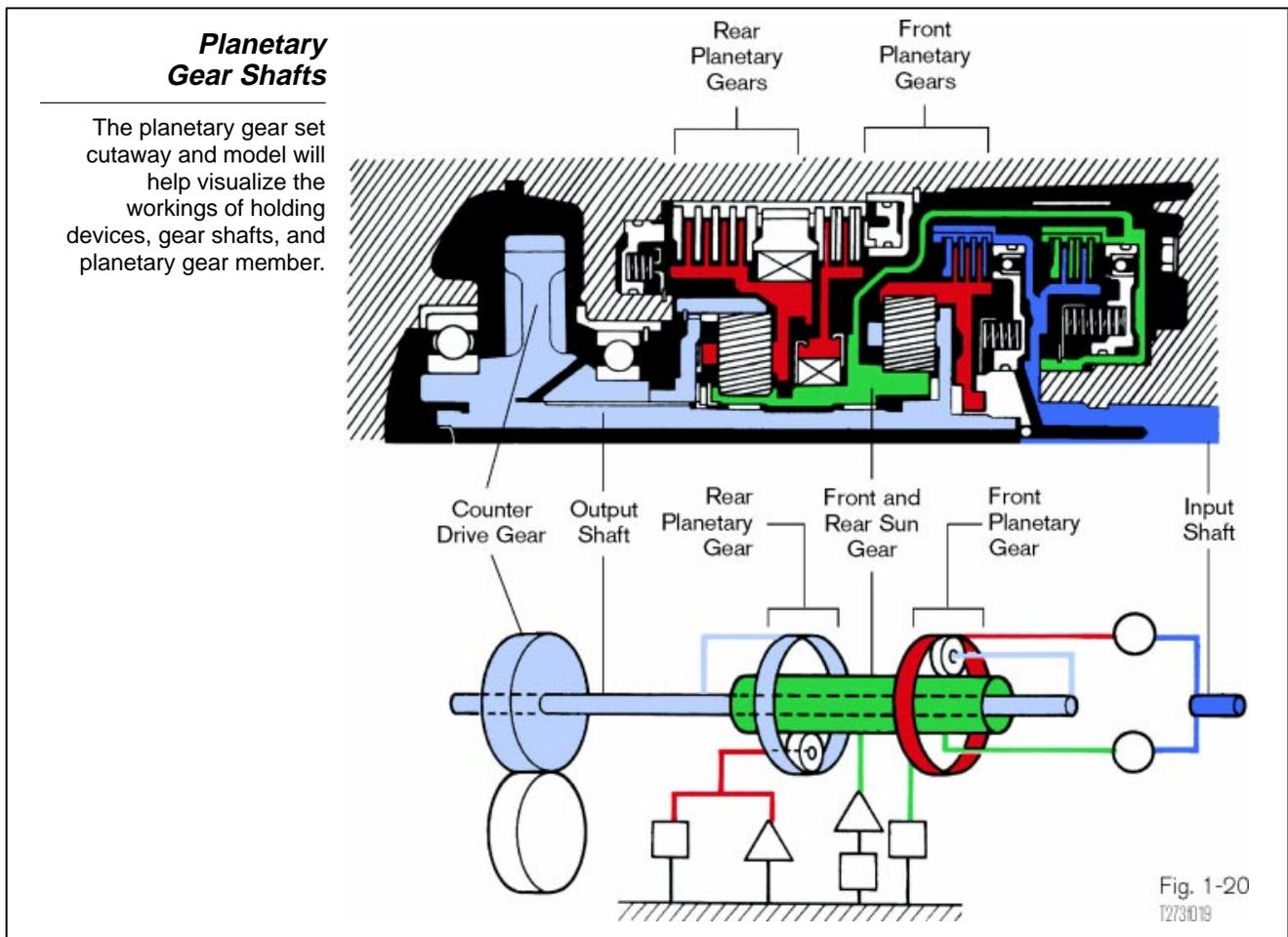
**Holding Devices** Multiplate clutches and brakes were discussed in detail earlier, and in the cutaway model on the next page, we can identify their position and the components to which they are connected. The holding devices for the Simpson planetary gear set are identified below with the components they control:
