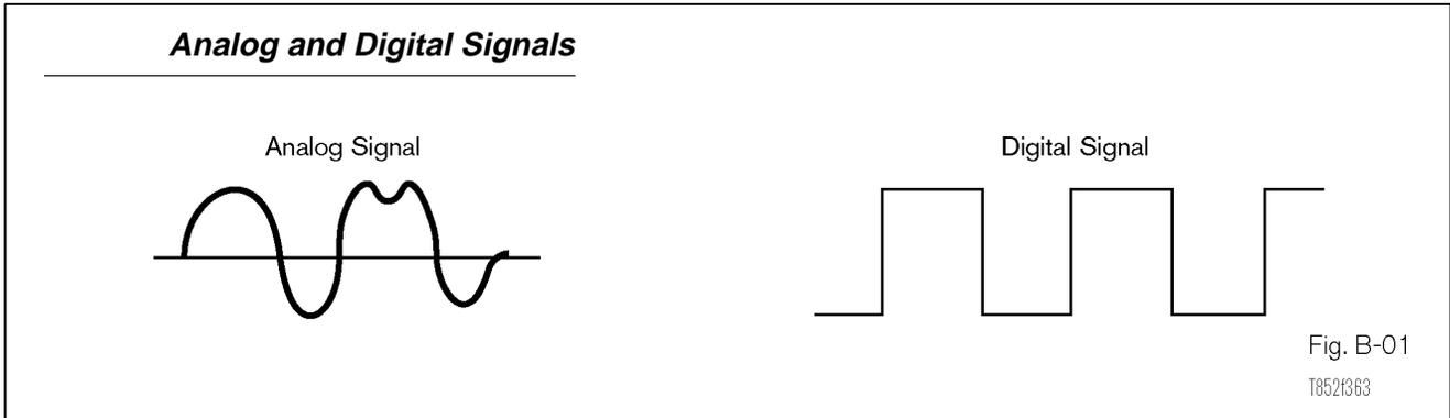
**Analog Signal** An analog signal is a variable signal and is usually measured by voltage or frequency. The voltage of the signal can be at any given point in a given range.
