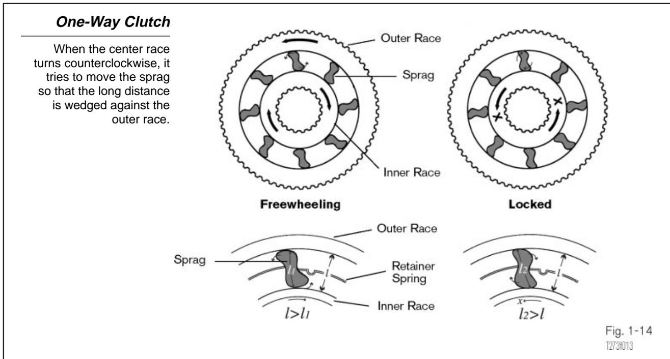
When the center race turns counterclockwise, it tries to move the sprag so that the long distance is wedged against the outer race. This causes the center race to stop turning. To assist the sprags in their wedging action, a retainer spring is installed which keeps the sprags slightly tilted at all times in the direction which will lock the turning race.
