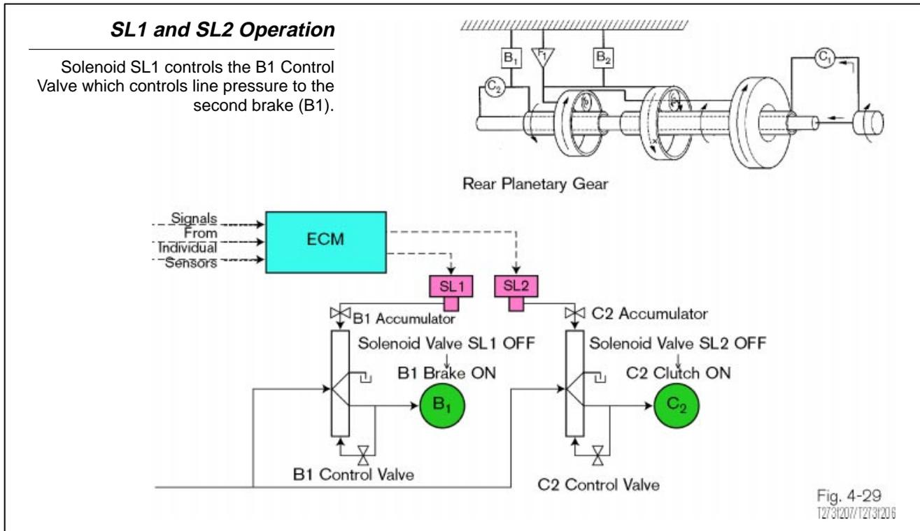
The *second brake* (B1) and the *direct clutch* (C2) both control the rear planetary sun gear. The shift from second gear to third requires the application of one holding device while the other is released. In an upshift to third gear, C2 connects the intermediate shaft to the sun gear while B1 releases the sun gear from the transmission case.
