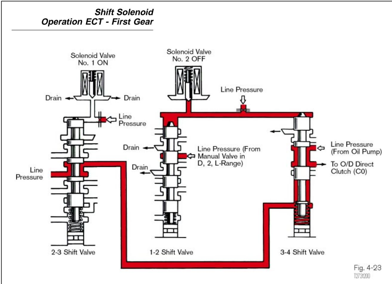
**First Gear** During first gear operation, solenoid No. 1 is ON and solenoid No. 2 is OFF. With line pressure drained from the top of the 2-3 shift valve by solenoid No. 1, spring tension at the base of the valve pushes it upward. With the shift valve up, line pressure flows from the manual valve through the 2-3 shift valve and on to the base of the 3-4 shift valve.
