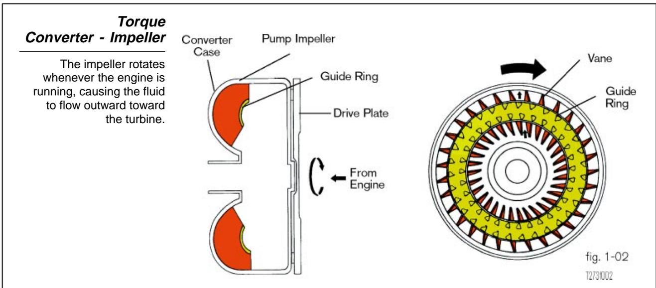
When the impeller is driven by the engine crankshaft, the fluid in the impeller rotates with it. When the impeller speed increases, centrifugal force causes the fluid to flow outward toward the turbine.
