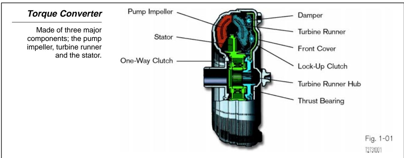
**Pump Impeller** The impeller is integrated with the torque converter case, with many curved vanes evenly spaced and mounted inside. A guide ring is installed on the inner edges of the vanes to provide a path for smooth fluid flow.
