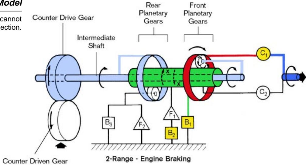
The sun gear is held in the counterclockwise direction only in a clockwise direction.
