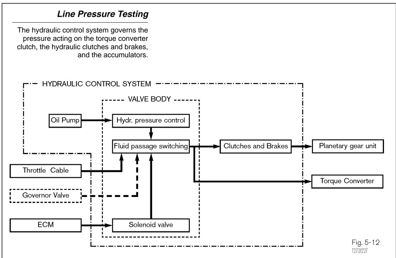
**Preparation** Prepare the vehicle for pressure testing by installing the high pressure gauge (0 to 300 psi) to the transmission. Refer to the vehicle’s repair manual for the test port location. When measuring line pressure at stall speed in the shop, be sure to chock all four wheels as a safety precaution.
