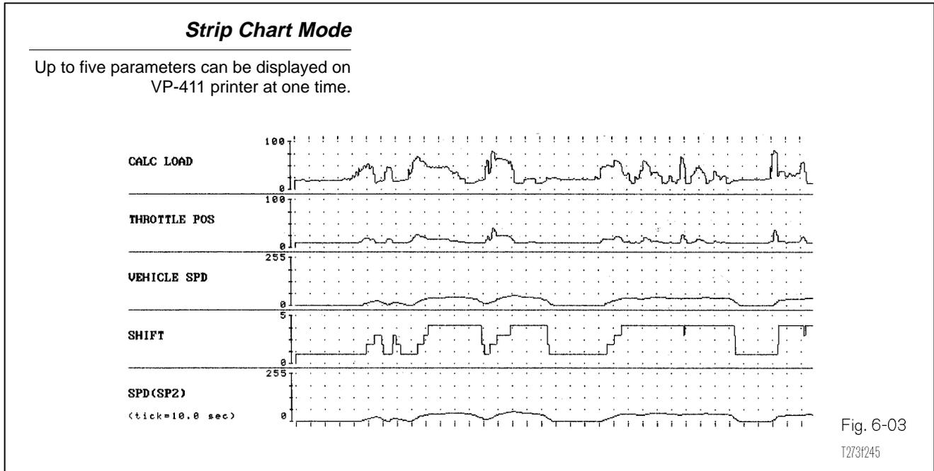
**Snapshot Features** The snapshot feature allows you to record data before and after a fault occurs. This provides for careful examination of all data parameters in the seconds just before and after the vehicle exhibits a driveability condition, or sets a diagnostic trouble code.
