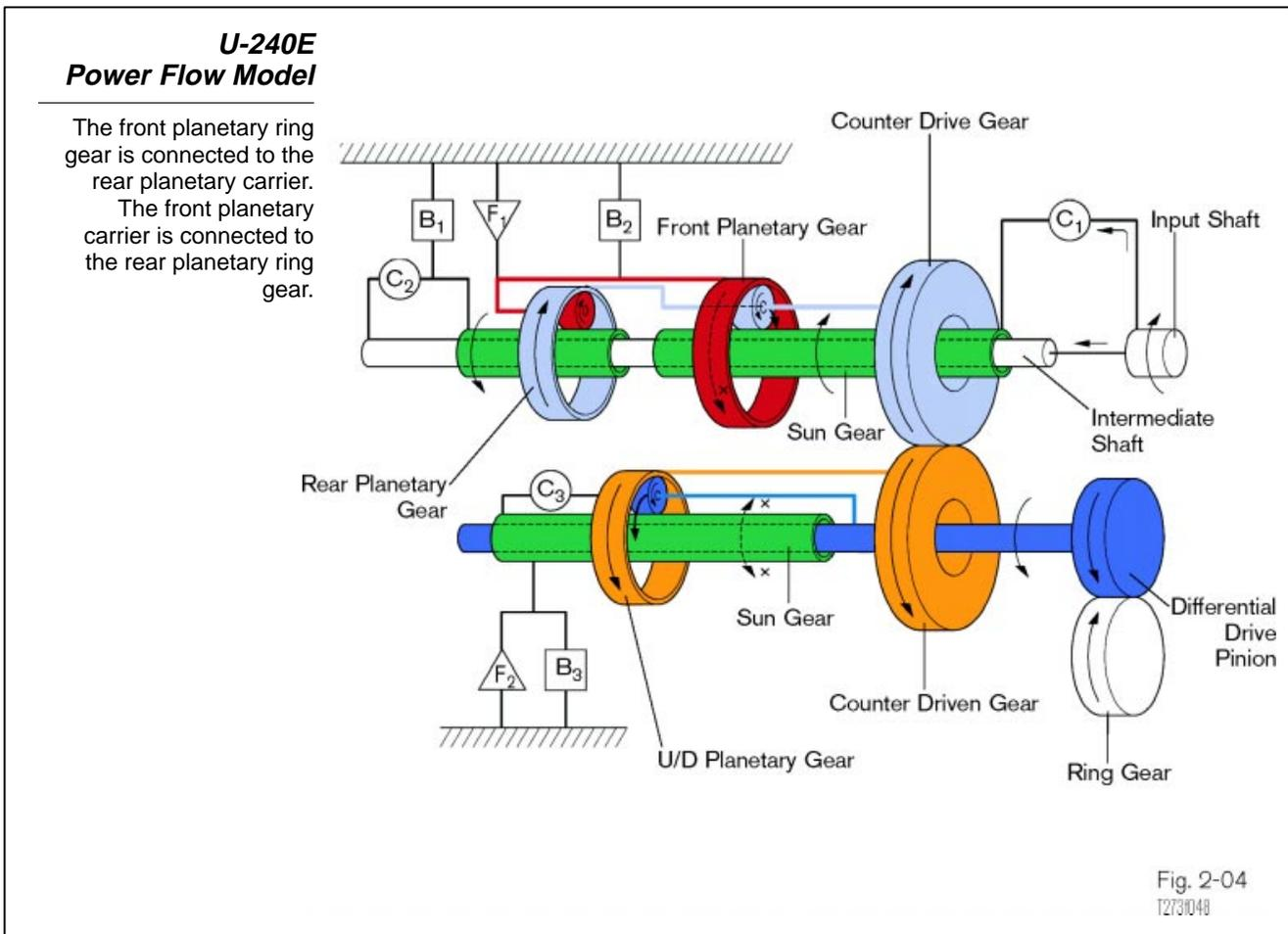
**Clutch/Brake Designation** The alphanumeric clutch designations (i.e. C1, B1, F1, etc.) have shared a common identifying name and function throughout the transmission model lines for many years. However, the U-series transaxles changed the identifying name as indicated in the shaded boxes in the chart below. For example, B2 has been known as the *2nd brake*, but is called *1st and reverse brake* in the U-240E and *2nd brake* in the U-341E.
